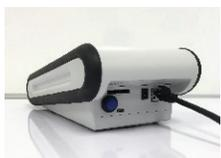
**01** Turn on the reader by pressing the button at the rear right-hand side of the back panel. As the instrument boots up, the Charles River logo will display on the touch screen.
