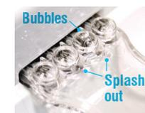
**14** Splash out will render the volume inaccurate, which can lead to invalid test results. Bubbles can cause false onset times due to the disturbance of light transmittance and can interfere with reconstitution of reagents within the cartridge.
